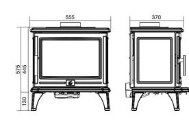
Long legs option: Overall height: 775mm • Floor to centre of rear flue: 650mm
